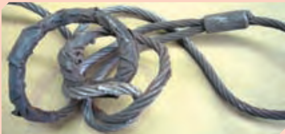
Examples of damaged flexible steel wire rope slings.
