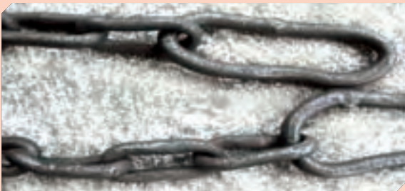
An ungraded chain showing effects of twisted links and stretched ring.
