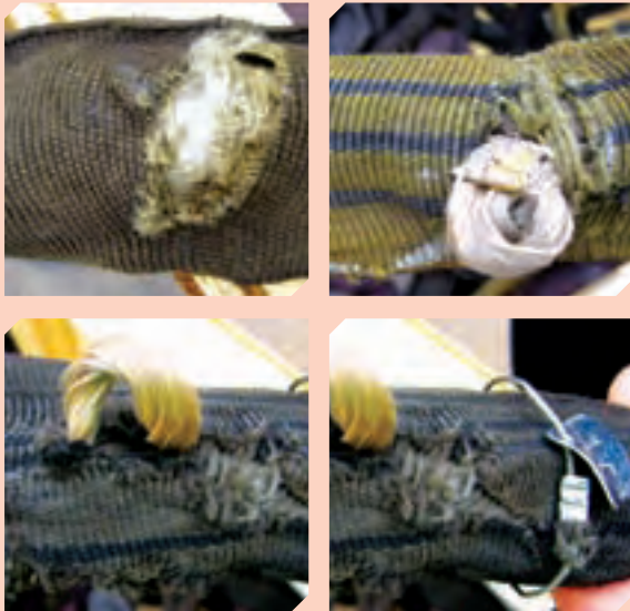
Examples of damaged synthetic slings.
